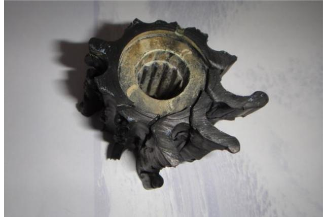
here. Probably better to do this when the engines are cool, but hey, I'm curious. Fortunately the pump on the starboard engine is somewhat accessible and the cover plate comes off easily. What I see tells me that I have found the problem with the cooling system. An impeller with most of the vanes missing will not pump water effectively!
